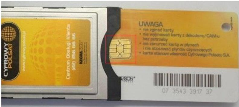
**Step2:** Loading QBOX CI with the CAM. The bumped side of the CAM and the brand-marked side of the QBOX should face the same direction. The CAM should be inserted in right way as follows so that it can work properly.
