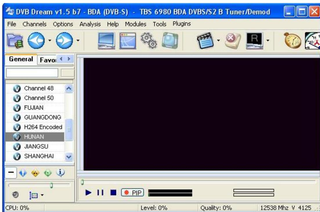
Click “Device” on “Options” menu. You can see TBS model name on the dialog. Some times, if device not started, you need to choose correct device from the up and down arrow and click “Start” to initialize device.
