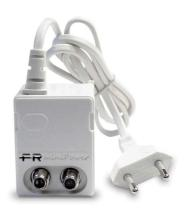
Miniaturized 24V stabilized switching type power supply withhigh efficiency and low consumption with 1 input, 1 output and 130mA delivered current. Type C plug for mains connection.
