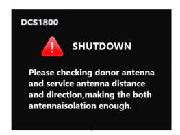
if not working and Self-oscillation get seriously, which overcome ISO and ALC function address range (ALC≥42dB, ISO≥42dB), the Sub-band (with Self-oscillation) would be auto-shutdown ass above message, which shows shutdown status (red) for this Sub-band in Menu Page, to protect Base Station wouldn't get interference.
